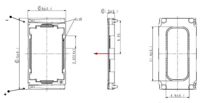
Positive voltage on pin '+' moves membrane in direction of red arrow!
